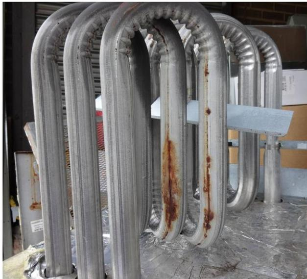
In this photo, condensate from the coils above the heat exchanger has dripped down onto the galvanized heat exchanger coils resulting in the rust and cracks you see here... cracks which could have leaked carbon monoxide! This Maytag residential gas/electric package unit was still under warranty when this was found, just 8 years after installation. Lucky for the homeowners, they did not succumb to carbon monoxide poisoning, and the warranty paid for the replacement of the heat exchanger.
